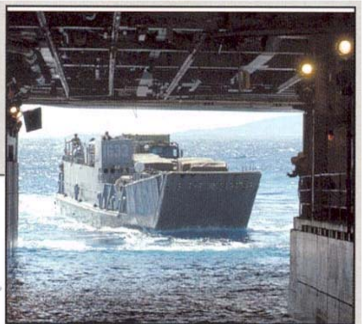
With the new LHDs an internal dock that landing craft can sail into will replace mating ramps. This technique is quick and easy and can be done in rough seas. Here a US Navy LCU enters the dock of an American amphibious ship.
