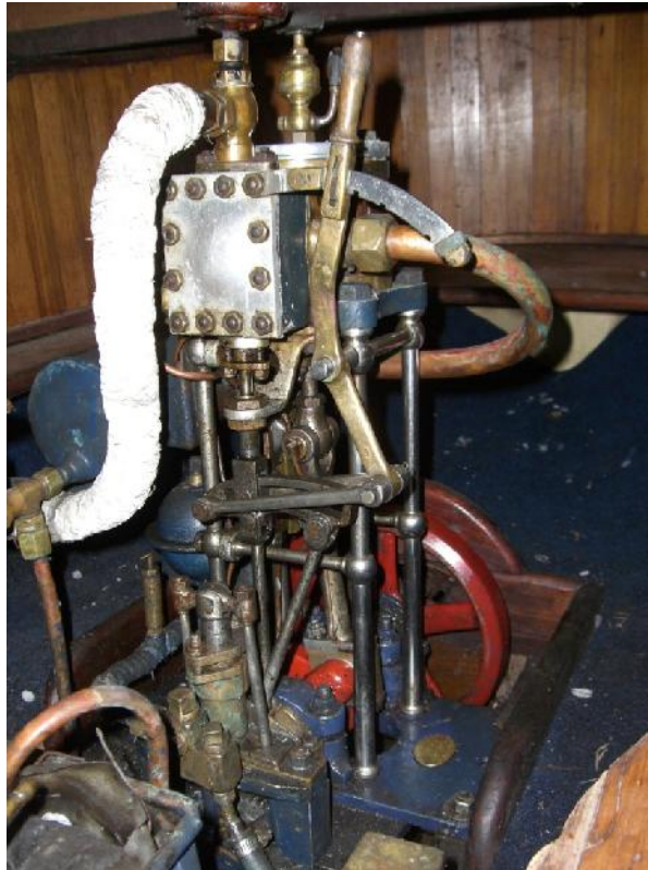
Steam engine made from a crankshaft and cylinder from a Honda.
